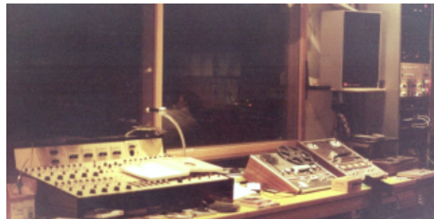
The recording studio with mixer, 2 and 4 track tape recorders and JBL control room monitor speakers
